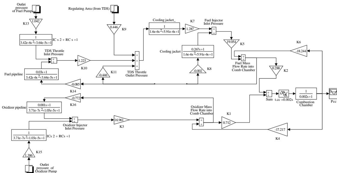
Figure 2 – Block diagram of the model considering the liquid compressibility
