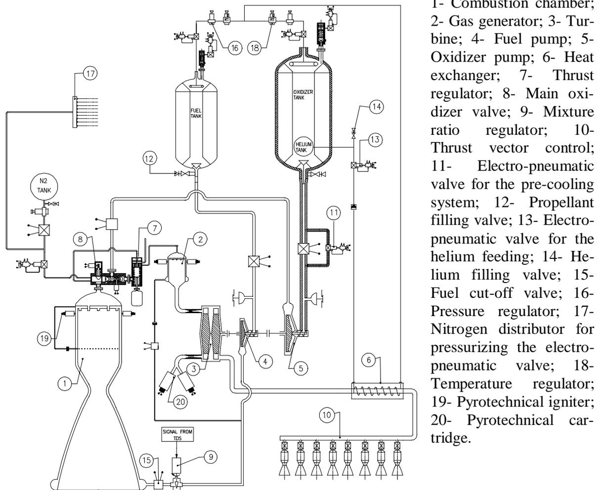
Figure 1- Hydropneumatic system of the rocket engine
