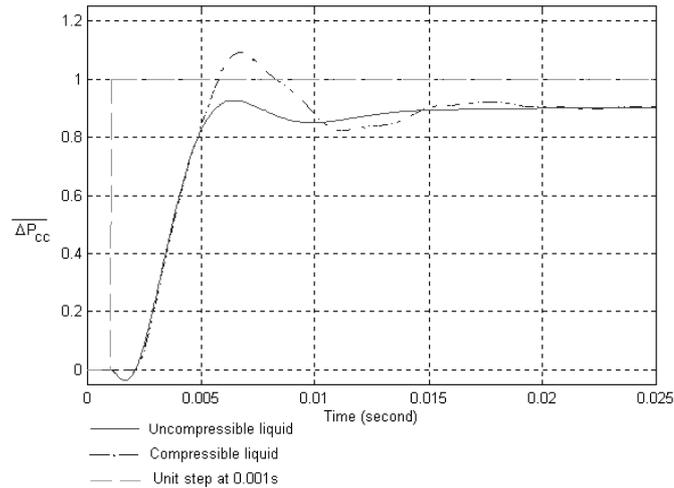
Figure 3- Comparison of the step response for the compressibility effect
