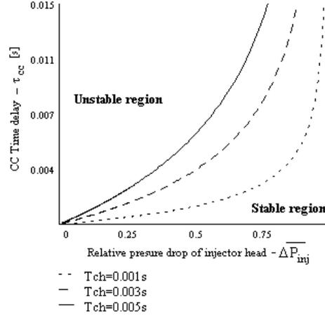
Figure 4- Boundaries of stability of combustion chamber for different values of  $T_{ch}$ .
